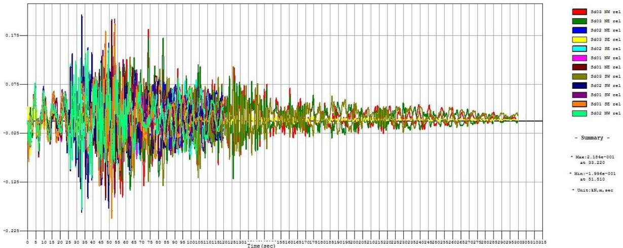
Figure 6. Opening (negative) and closing (positive) of the gaps, in metres, between the truss ends at the tower bearings for the subduction interface records.
