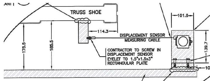
Figure 9. Location of the displacement sensor on bearings.
