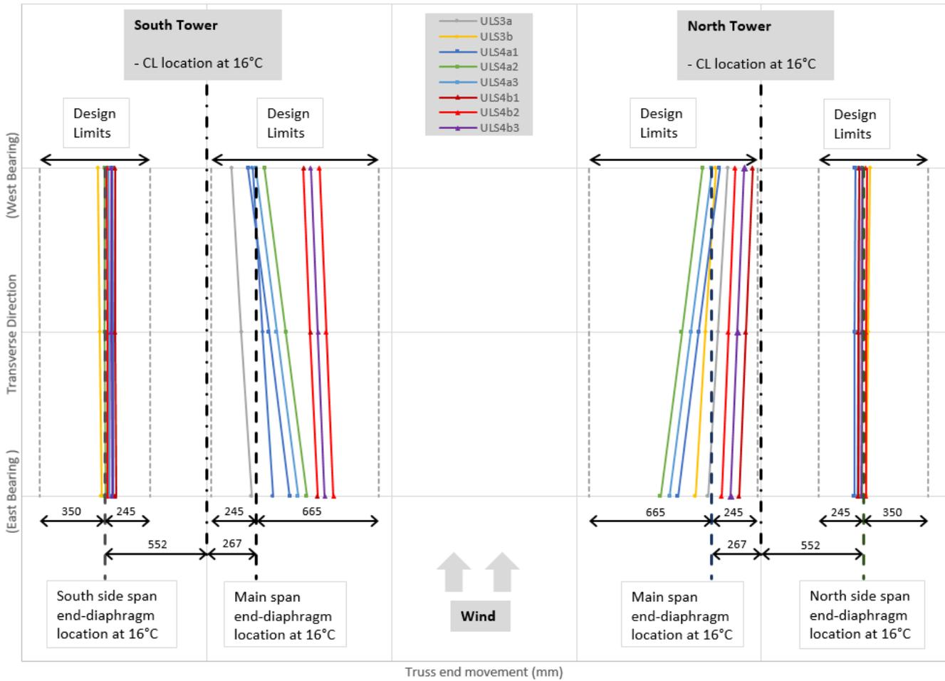
Figure 5. Longitudinal bearing displacement from static loads cases.
